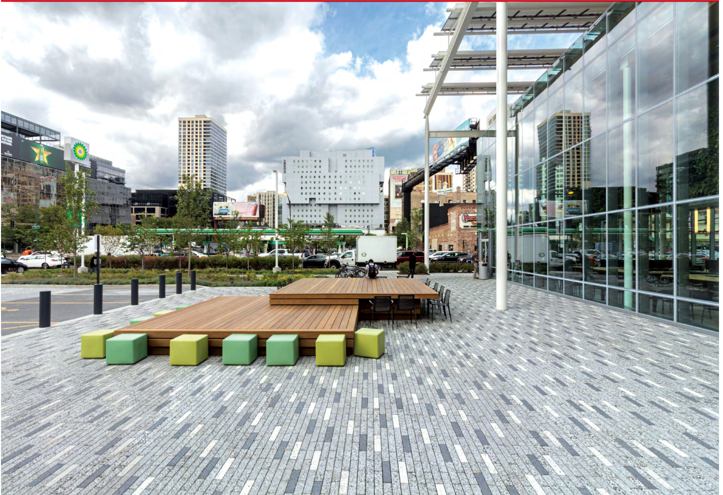
McDonald's Chicago Flagship in Chicago IL. Designed by Ross Barney Architects | Product: Series™ Permeable Pavers, Size: 3 x 12 (3 7/8"), Color: 3 Custom Colors
