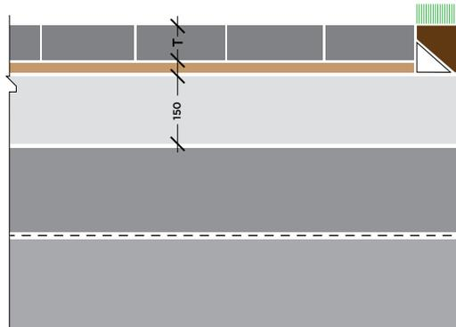
Concrete paver installation resulting in 60% concrete material savings and 25% embodied carbon savings.
