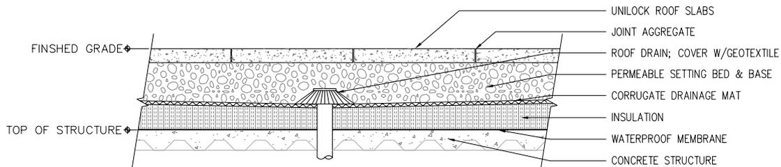
The cross sections shown are examples of the type of installation systems and technical features of Unilock products. Unilock shall not be deemed responsible for improper use of the product or of damage deriving from any use different from those recommended
