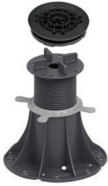
Self-leveling head provides for slope compensation up to 7%, keeping paver slabs level on a sloping surface.
