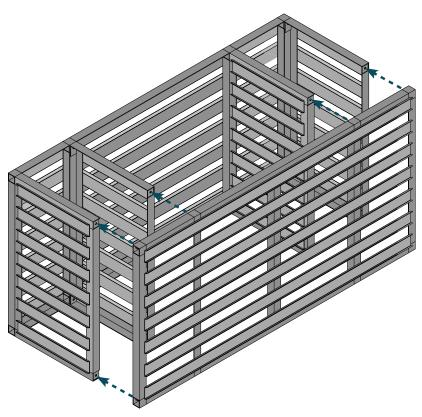
ATTACH THE FRONT PANEL USING INCLUDED HARDWARE AND SECURELY TIGHTEN ALL BOLTS
