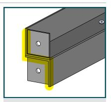
Once completed, there will be 2 mounting sides to allow for attachment to cabinet and for interior rail cut-out.
