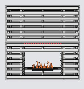
HEAT RATED SEALENT/CAULK SHOULD BE USED FOR ANY OPEN GAPS AROUND THE PERIMETER OF THE HEATSHIELD.
