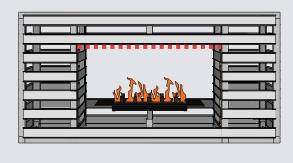
HEATSHIELD MUST BE GLUED TO TOP OF FASCIA PANEL USING HEAT RATED ADHESIVE.
