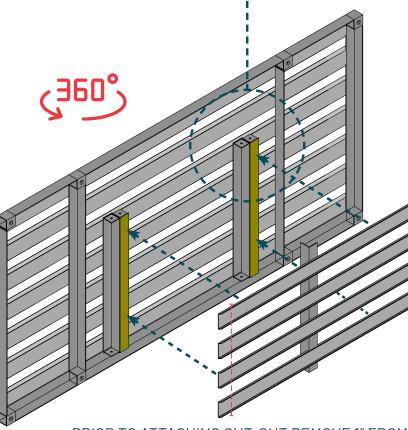
PRIOR TO ATTACHING CUT-OUT REMOVE 1" FROM EITHER END TO ALLOW FOR CLEARANCE
