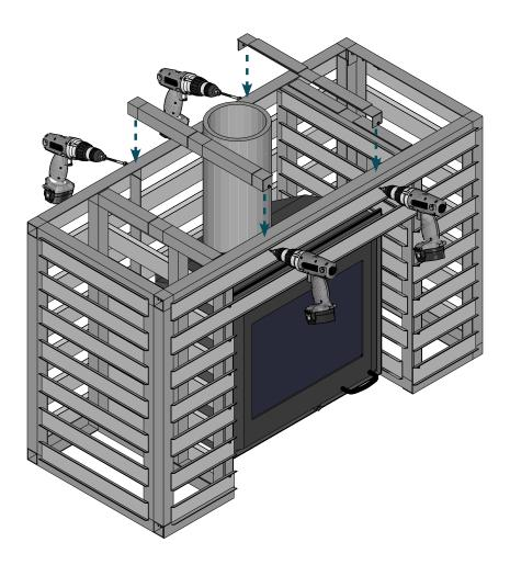
ADJUST HAR ON BOTH SIDES OF THE FLUE PIPE TO HELP KEEP IT ALIGNED. THESE WILL BE TUCKED UNDER THE TOP ANGLE RAIL.
